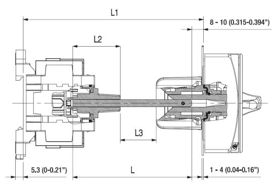
To determine the cut length L of the shaft, consider the following guidelines: L3  $\ge$  1mm 12mm  $\le$  L2  $\le$  32mm
