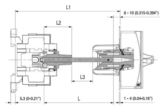
To determine the cut length L of the shaft, consider the following guidelines:
